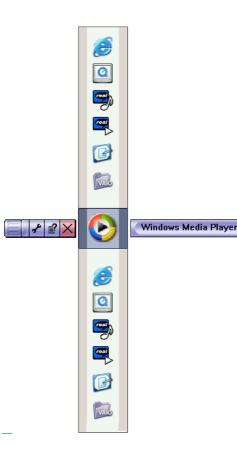
Rotate the Jog Dial™ wheel up and down to view the software applications and utilities on your computer. To launch an application, make sure it is selected and press the Jog Dial™.
